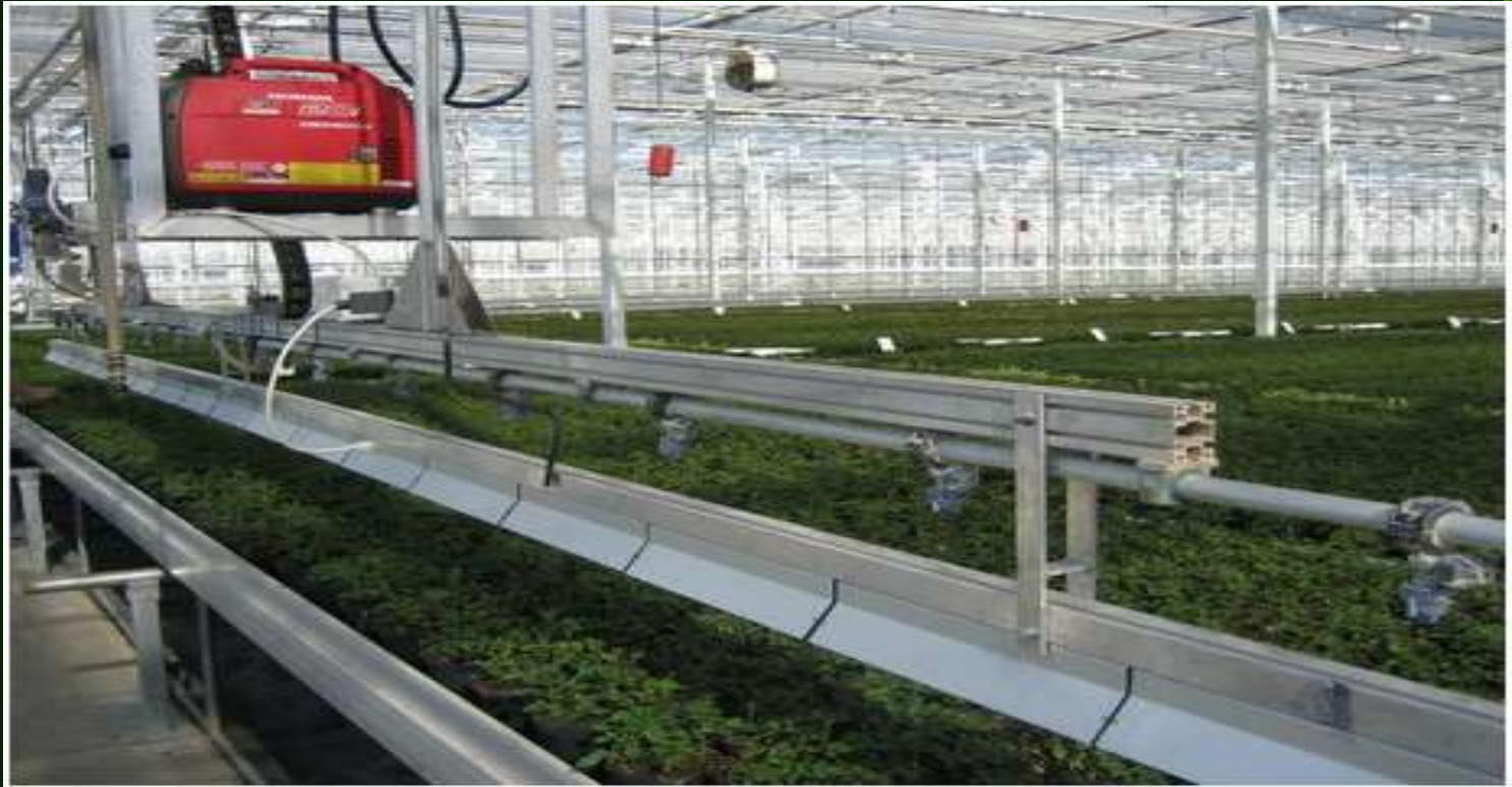
UV light: effective treatment against powdery mildew
